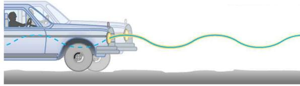
**Figure 16.10** The bouncing car makes a wavelike motion. If the restoring force in the suspension system can be described only by Hooke's law, then the wave is a sine function. (The wave is the trace produced by the headlight as the car moves to the right.)
