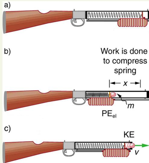
**Figure 16.7** (a) In this image of the gun, the spring is uncompressed before being cocked. (b) The spring has been compressed a distance  $x$ , and the projectile is in place. (c) When released, the spring converts elastic potential energy  $PE_{el}$  into kinetic energy.
